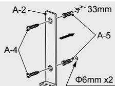
When mounting on a plaster board or tiled wall.
